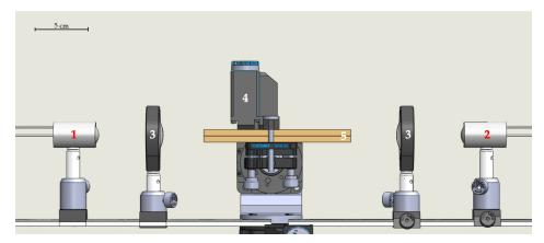
**Figure 3.** Side view of the opto-mechanical setup utilized for the measurements: (1) emitter, (2) detector, (3) TPX collimating lenses, (4) micrometric alignment system, (5) waveguide with embedded antennas.
