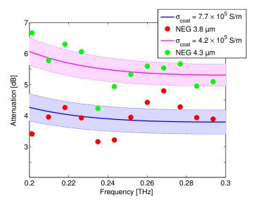
**Figure 6.** Experimental relative attenuation as a function of frequency on the NEG coated slab of 3.8  $\mu$ m and 4.3  $\mu$ m (red and green dots respectively) and best fit curves (blue and magenta lines respectively).
