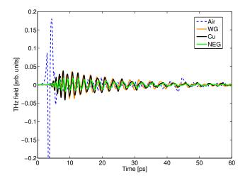
**Figure 4.** THz time domain averaged signal propagating in air (dashed line), through the waveguide without (orange, continuous line) and with copper (black, continuous line) or NEG coated (green, continuous line) slab.
