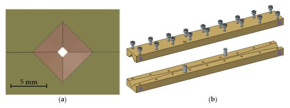
**Figure 2.** Sketch of the device used for the spectroscopy measurements, consisting in a diagonal section waveguide ending with two pyramidal horn antennas. (a) Front view of the assembled device; (b) open view of the waveguide and the embedded antennas. The overall size of the device is  $16 \times 12 \times 140 \text{ mm}^3$ .
