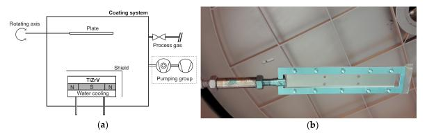
**Figure 1.** Non-evaporable getter (NEG) deposition setup. (a) Drawing of the system; (b) detail of the copper slab placed in the aluminum frame. The four holes shown in the picture are used for the alignment in the waveguide during THz measurements.
