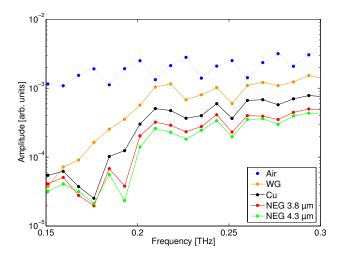
**Figure 5.** Frequency spectrum showing the averaged amplitude transmission data in air (dashed line-to-point curve), through the waveguide without (orange line-to-point curve) and with copper (black line-to-point curve) or  $3.8~\mu m$  and  $4.3~\mu m$  NEG coated (red and green line-to-point curves respectively) slabs.
